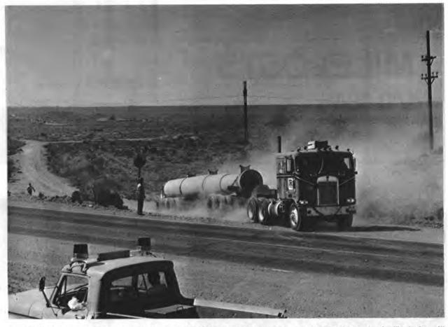
59 TONS of gun barrel leave Sandia for Oblivion. With an equal-sized partner, it served as a test facility in Area III since the mid-fifties. Originally from the Naval Gun Factory, the 45-foot barrels were bored out to a 26-inch diameter and used both as a pressure vessel and as an explosive gas shock tube. Subroc missile, now in the fleet, was its biggest test. Here it's a test of traction and power as a contractor/purchaser eases the big barrel across Tijeras Arrovo.
